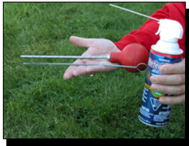
Figure 4—It is important to clean the hole thoroughly to prevent misfires. The BMS Micro-Blaster comes with a bore brush and hand-pumped bulb blower. A can of compressed air also works well.
