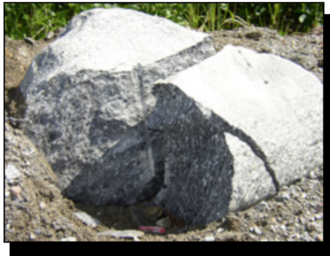
Figure 9—Another rock broken with a BMS Micro-Blaster shot using a single cartridge. The spent cartridge is at the base of the rock.
