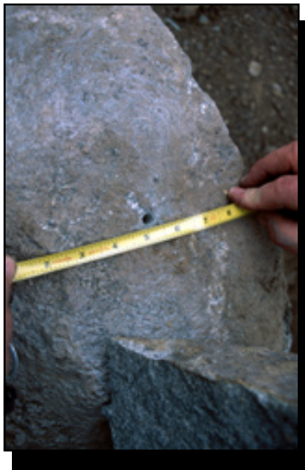
Figure 3—The size of the hole in the rock is important. Holes must be drilled straight using a carbide-tipped, \frac{5}{16} -inch masonry bit.
