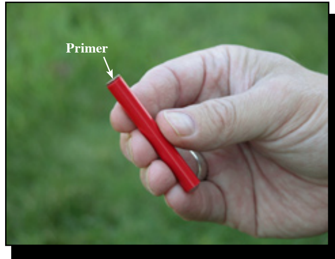
Figure 2—The BMS Micro-Blaster cartridge is about the same diameter as a .32-caliber shell but has explosive properties similar to those of a cartridge as large as a shotgun shell. The brass cap on one end of the cartridge is the primer.
