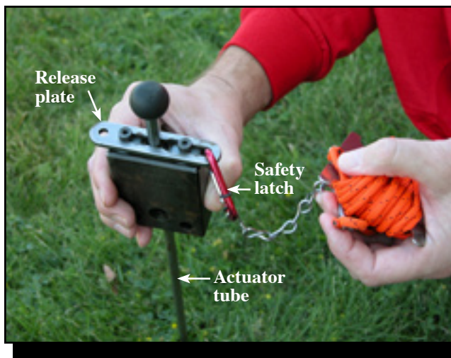
Figure 1—The BMS Micro-Blaster shown in fully cocked position with the safety locked in place and a 25-foot lanyard attached.
